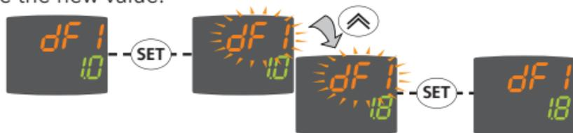
**NOTE:** It is advisable to switch the instrument off then back on again each time parameters are modified to prevent malfunction of the configuration and/or timer operations underway.
