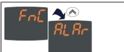
After pressing the **fnC** key, you can scroll through the two folders in the menu (FnC and ALAr) using the **⏪** and **⏩** keys.
