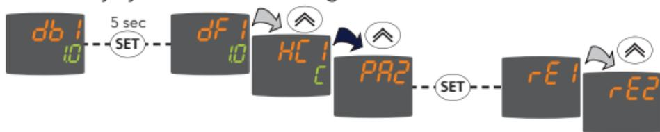
Press the **set** key next to the desired folder ("rE2" in the example), the first parameter contained in the folder will be displayed. Select the desired parameter using the **⏮** and **⏭** keys. Change the value (shown on the second line) using the **⏮** and **⏭** keys, then press the **set** or **fnc** keys to store the new value.
